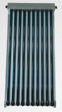
Evacuated tube collector of 727 W output (at 1000 W/m<sup>2</sup> irradiance), designed for on-roof portrait installation. A tube consists of 2 coaxial glass tubes with vacuum between them. An aluminum lamella fitting closely to the glass tube collects heat from the whole inner surface of the evacuated tube, giving it away into solar fluid inside the copper pipe. These copper pipes join the collector header, insulated with 30 mm of mineral wool.
