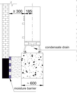
Water condensation normally occurs during heat pump operation; up to 50 liters of condensate can be generated per day, depending on the operating conditions.
