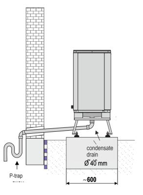
It is recommended to insulate the outdoor section of drain pipe with thermal insulation.
