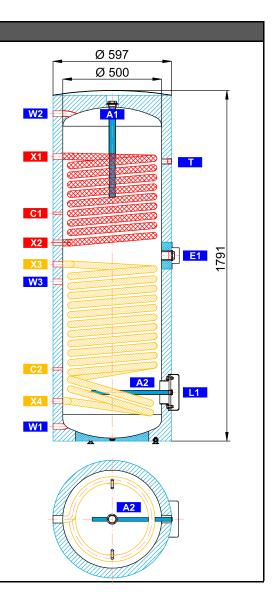
C1 and C2 tappings are supplied incl. adapter G 1/2" M - M12x1.5 and cable gland
