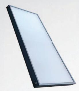
Flat plate collector designed for on-roof portrait installation. A harp absorber with highly selective TiNOx surface is laser welded to the copper pipes. The insulation consists of 40mm mineral wool. Connections are located on both sides on the top and bottom.
