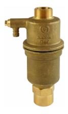
In order to remove air from the circuit perfectly, the pump station is equipped with a so-called air separator with an air vent valve. After filling or topping up the fluid in the circuit and during the pre-season check, it is always recommended to release the air using the air vent valve.
