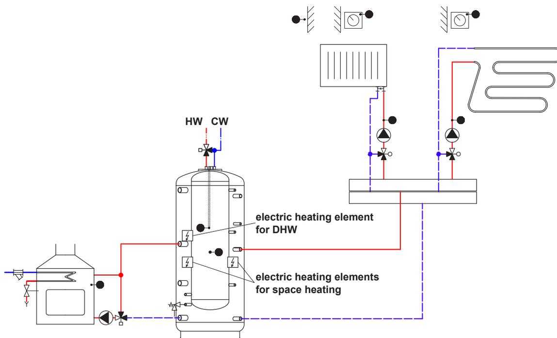
**Hydraulic variant 2: Fireplace combined with a switched boiler (gas fired, electric fired..)**
