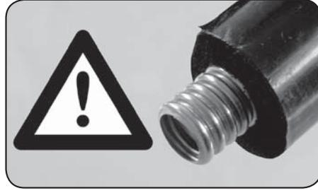
Check the cut pipe and remove any possible burrs.
