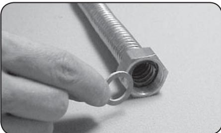
Insert the gasket and check for proper position of the lock ring.
