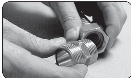
Turn in the appropriate fitting into the connecting nut (for example: fitting with external thread x compression fitting).
