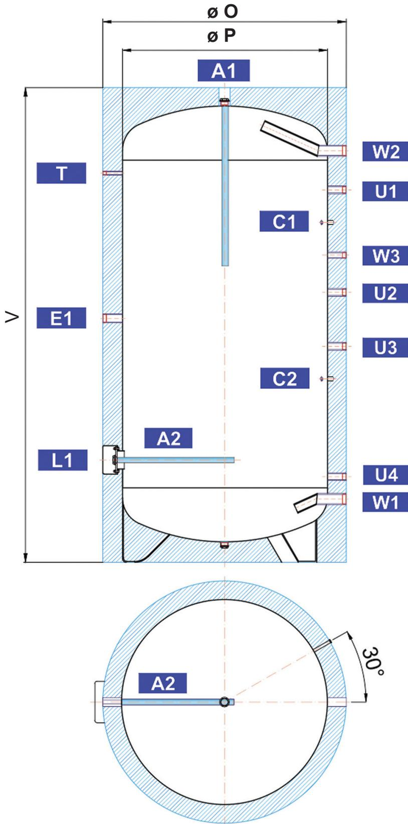
The lower flange contains an anode rod in tanks: R0BC 1500 - R0BC 3000
