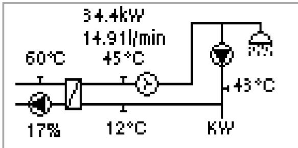
The graphics or overview mode appears when no key has been pressed for 2 minutes, or when the main menu is exited by pressing “esc”.
