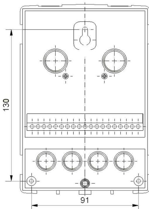
5. Using a drill and size 6 bit, drill 3 holes at the points marked on the wall and push in the plugs.
