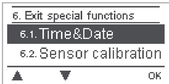
Menu “6. Special functions” is used to set basic items and expanded functions.
