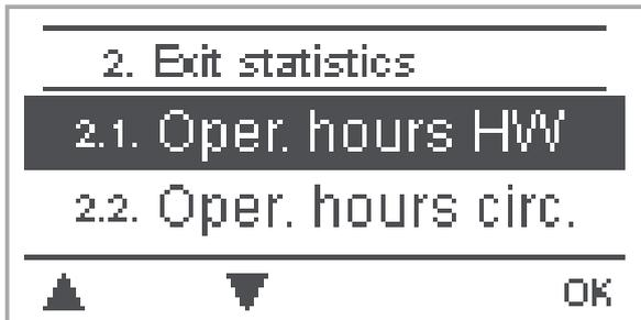
The menu “2. Statistics” is used for function control and long-term monitoring of the system.
