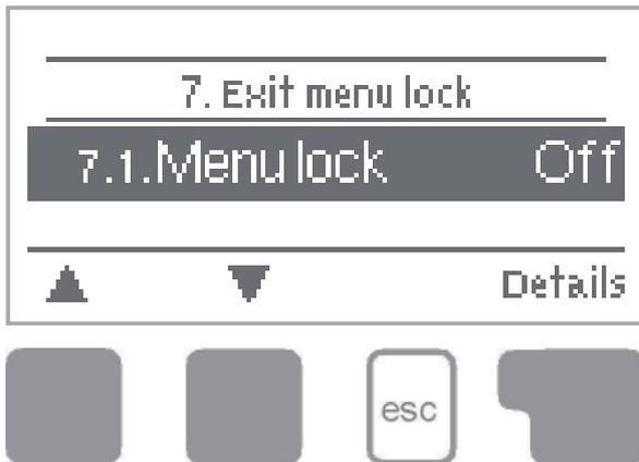
Menu “7. Menu lock” can be used to secure the controller against unintentional changing of the set values.
