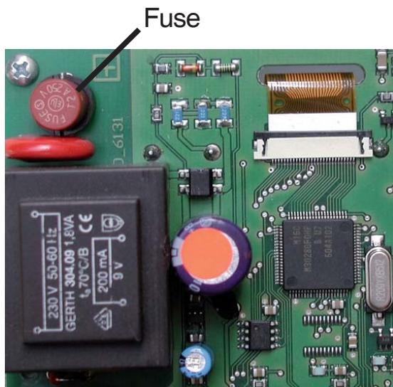
If the mains voltage is switched on and the controller still does not function or display anything, then the internal device fuse may be defective. In that case, open the device as described under 3.1, remove the old fuse and check it.
