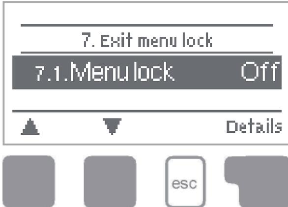
Menu “7. Menu lock” can be used to secure the controller against unintentional changing of the set values.
