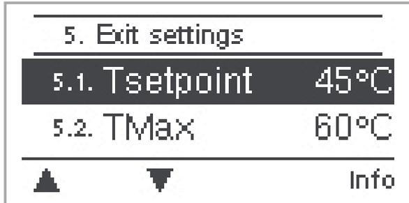
The necessary basic settings required for the control function are made in menu “5. Settings”.
