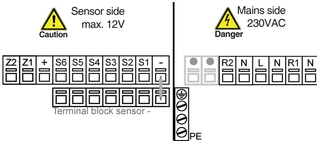
**Low voltage** max. 12VAC/DC connection in the left-hand terminal compartment!
