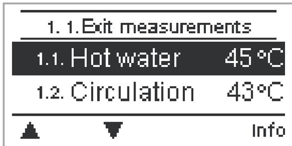
The menu “1. Measurement values” serves to display the currently measured temperatures.
