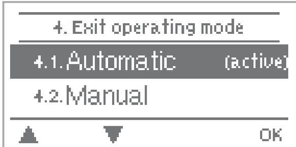
In menu “4. Operating modes” the controller can either be placed in automatic mode, switched off, or placed in a manual operating mode.
