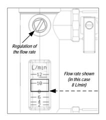
**(3)** - Regulate the flow rate using the regulation rod until the right flow rate is shown.
