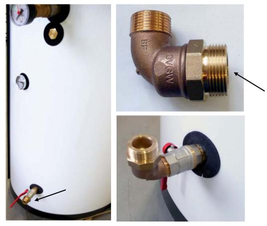
5. Remove the plug below the pressure gauge assy and fit the zone valve connection assy (code 13967) in its place. Remove the handle from the assembly prior to fitting and then return it back.
