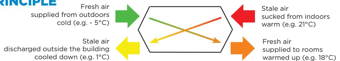
Fresh air is sucked into the HRV unit either through an outer wall or through a vent duct termination in a roof. The incoming fresh air flows into the HRV unit where it is preheated in a heat exchanger by heat taken from the warm stale exhaust air.
