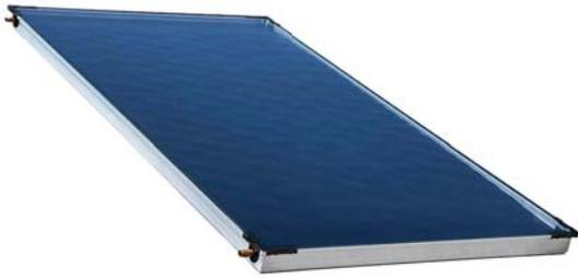
Flat plate solar collector of 1882 W output (at 1000 W/m<sup>2</sup> irradiance) designed for either portrait or landscape on-roof installation. A harp absorber with highly selective TiNO<sub>x</sub> surface is laser welded to copper tubing. The insulation consists of 40 mm mineral wool. Connection points are located laterally on the top and bottom.
