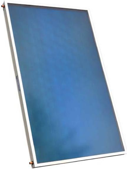
Flat plate collector of 1802 W output (at 1000 W/m<sup>2</sup> irradiance), designed for on-roof portrait installation. A harp absorber with highly selective TiNOx surface is laser welded to the copper pipes. The insulation consists of 40 mm mineral wool. Connections are located on both sides on the top and bottom.
