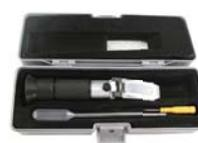
**Manual Refractometer** (frost protection measurer) for freezing point measurement of anti-freeze fluids.
