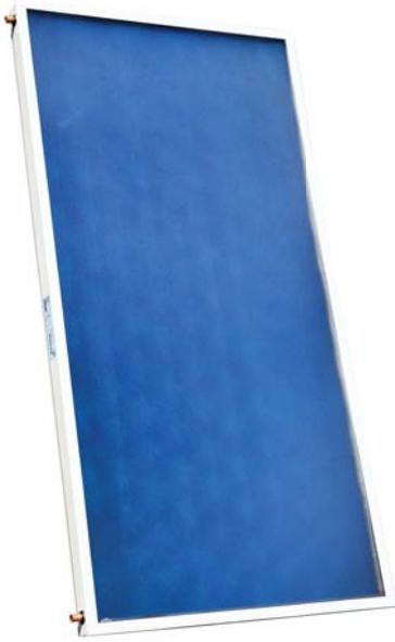
Flat plate collector of 1481 W output (at 1000 W/m<sup>2</sup> irradiance), designed for on-roof portrait installation. A harp absorber with highly selective TiNOx surface is laser welded to the copper pipes. The insulation consists of 40 mm mineral wool. Connections are located on both sides on the top and bottom.
