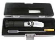
**402 ATC Refractometer** for freezing point measurement of antifreeze fluids.
