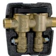
**Filling manifold for primary** circuits with two-way valves, filter, fill/drain valves and insulation, intended for filling, flushing and air discharging.
