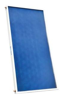
Flat plate collector of 1481 W output (at 1000 W/m² irradiance), designed for onroof portrait installation. A harp absorber with highly selective TiNOx surface is laser welded to the copper pipes. The insulation consists of 40 mm mineral wool. Connections are located on both sides on the top and bottom.
