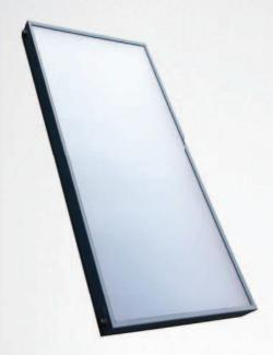
Flat plate collector designed for on-roof portrait installation. A harp absorber with highly selective TiNOx surface is laser welded to the copper pipes. The insulation consists of 40 mm mineral wool. Connections are located on both sides on the top and bottom.
