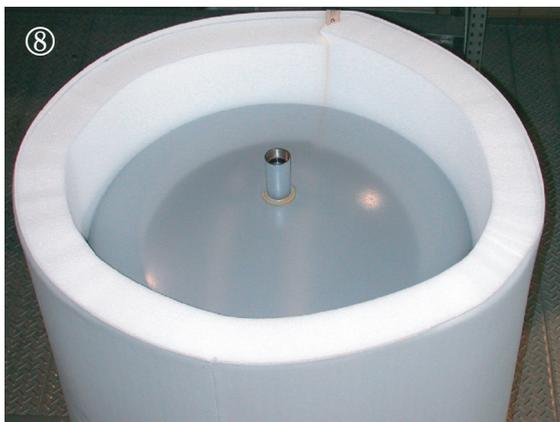
Pictures showing how to mount soft-foam insulation with a PVC sheet on a tank.
