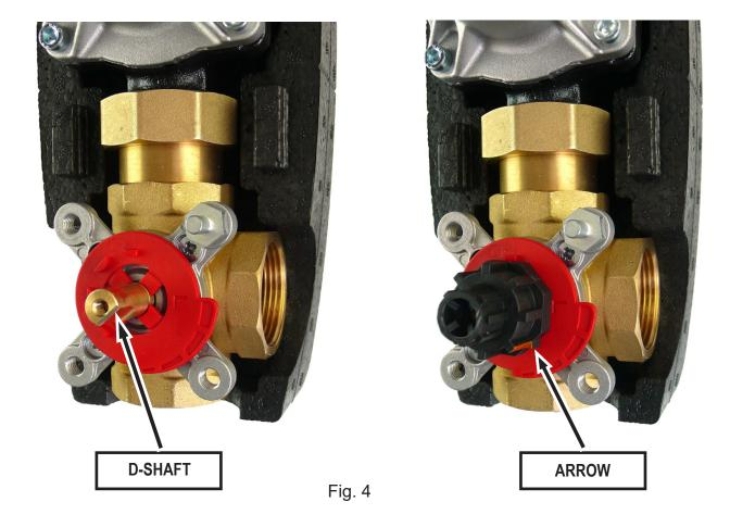
Prior to fitting the actuator on the plastic adapter, switch it to manual control, set the control knob to the middle of its control range and then fit the actuator onto the adapter already on the valve. The control knob shall be able to turn freely both to left and right by 45°. When turned to the right by 45°, the path 1 is closed, and when turned to the left by 45° the path 3 is closed. Having performed the check, turn the knob back to automatic control.
