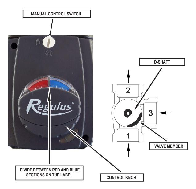
After the actuator is fitted, the correct position of the round indication label (hot/cold, red/blue) shall be checked as to the right function and position of the valve; the colours shall correspond to the cold and hot water connections. In case of a vertical installation in central heating, the red mark on the label shall be on the right-hand side for left-hand installations (see Fig. 5) and on the left-hand side for right-hand installations (see Fig. 5).
