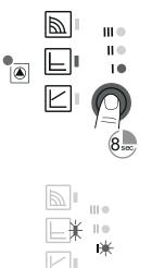
To lock the operating button, press it for 8 seconds.
