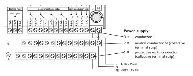
The power supply to the controller must be effected by an external power switch (last procedure) and the supply voltage must be 210 ... 250 Volt (50 ... 60 Hz). Flexible lines must be fixed at the housing or in a cable conduit (see tip
