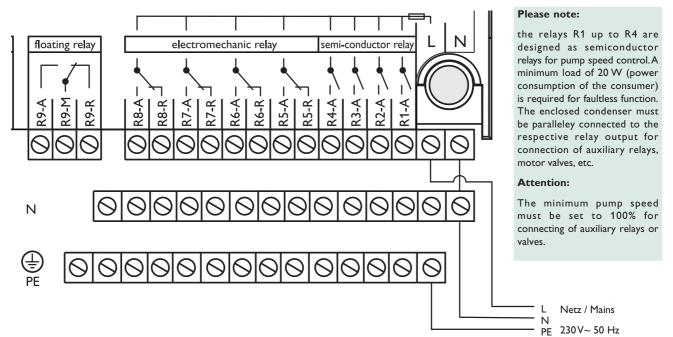
The controller is totally equipped with 9 relays, to which the **consumer** (actuators), e. g. pumps, valves, mixer and auxiliary relays can be connected:
