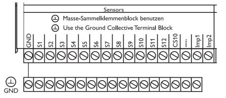
The controller is totally equipped with 15 sensor inputs. The earth connection for sensors is effected by the earth terminal strip (GND).
