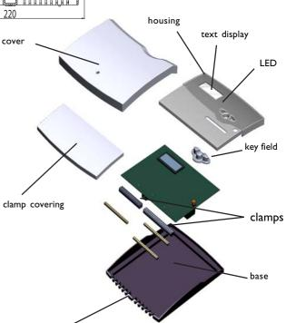
cable conduits with strain relief
