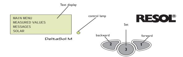
The controller is only operated by the 3 pushbuttons beside the display. The forward-button (1) is used for scrolling forward through the menu or to increase the adjustment values. The backward-button (2) is accordingly used the other way round. Button 3 is used for selection of the menu lines and confirmation.
