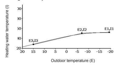
The controller calculates the desired heating water temperature with respect to the outdoor temperature and the 2- or 3-point heating curve. Using a 3-point curve is recommended that should precisely represent the insulation qualities of the building. Should the value of I3 be zero, the controller will use just a line through points E1, I1 and E2, I2.
