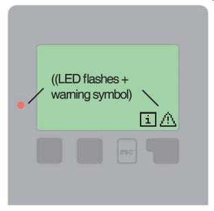
If the controller detects a malfunction, the red light flashes and the warning symbol also appears in the display. If the error is no longer present, the warning symbol changes to an info symbol and the red light no longer flashes. To obtain more detailed information
