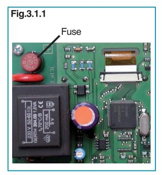
If the mains voltage is switched on and the controller still does not function or display anything, then the internal device fuse may be defective. In that case, open the device as described under 3.1, remove the old fuse and check it.
