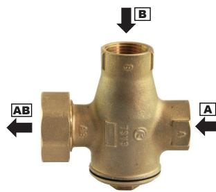
The TSV3B load valve is fitted with an integrated thermostatic insert that will close the A inlet (from a heating system), if the return water temperature to the boiler (AB outlet) is lower than the opening one. As soon as the opening temperature is reached, the thermostat starts opening the A inlet slowly and mixing the cold return water with the hot water from the B inlet (boiler flow) with the aim to reach the opening temperature (AB outlet) in the return pipe.
