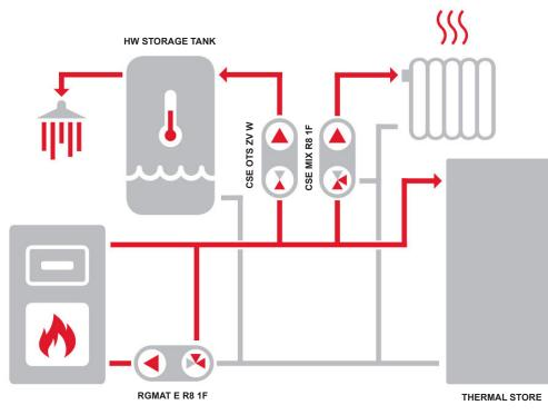
The diagram shows a typical connection of a solid fuel boiler, thermal store and heating circuit (with the recommended CSE MIX R8 1F pump station – not included in supply). If the boiler is used also for hot water heating, it is recommended to install a CSE OTS ZV W pump station (not included in supply).
