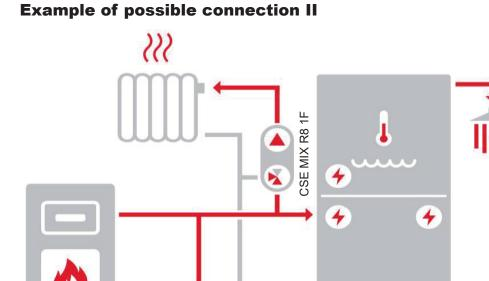
The diagram shows a typical connection of a solid fuel boiler, combination thermal store and heating circuit (with the recommended CSE MIX R8 1F pump station – not included in supply).
