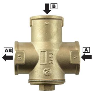
The TSV5B oad valve is fitted with an integrated thermostatic insert that will close the "**A**" inlet (from a heating system), if the return water temperature to the boiler ("**AB**" outlet) is lower than the opening one. As soon as the opening temperature is reached, the thermostat starts opening the "**A**" inlet slowly and mixing the cold return water with the hot water from the "**B**" inlet (boiler flow) with the aim to reach the opening temperature ("**AB**" outlet) in the return pipe.
