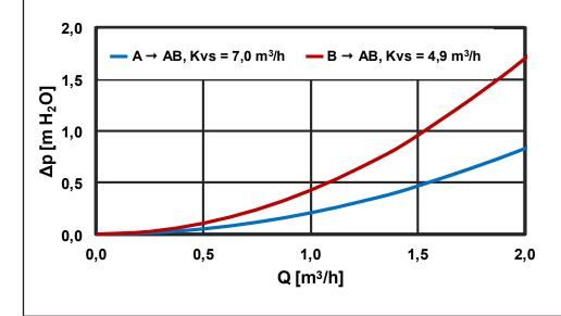
The pressure drop value moves between the two curves depending on the mixing ratio during mixing.
