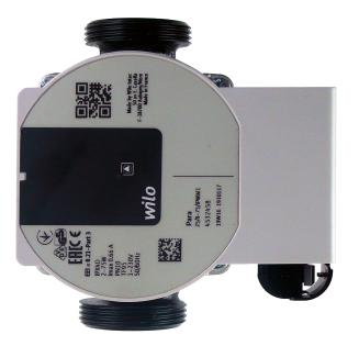
6.2. Permitted and Prohibited Pump Positions The Wilo Para 25/8 iPWM1 is a wet running circulation pump. The pump speed is controlled by the PWM signal. When the PWM signal is disconnected, the pump runs at its maximum speed. The operating status and possible faults of the pump are indicated by LEDs directly on the pump. The pump is able to send the current flowrate electronically to an external controller. The controller must be equipped with an iPWM read input and a flow calculation function.
