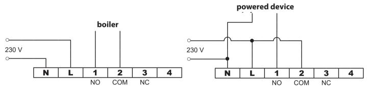
The voltage at terminals 1 and 2 depends solely on the system to be controlled, so the cable cross-section must respect the type of device controlled by the thermostat. The length of the cables does not play any role, the receiver can be placed near the boiler or far from it, but never under its casing.
