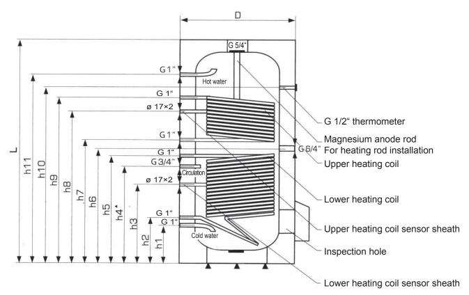
Openings for a heating rod and thermometer are located opposite the other ones.
