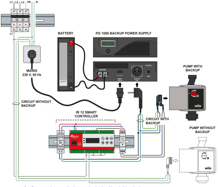
Do respect the separation between the circuits with and without backup. Not only for the live wire but also for the neutral one!
