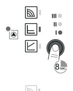
To lock the operating button, press it for 8 seconds.
