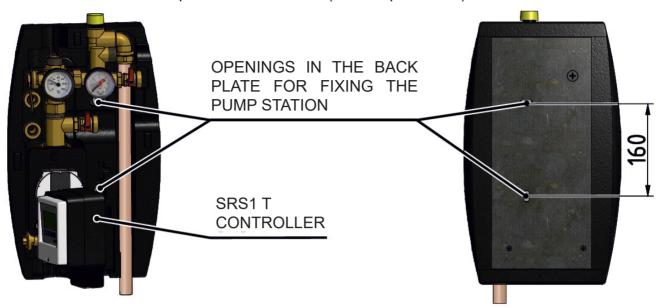
The supply involves an installation kit that is used to fix the pump station in its place.
