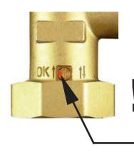
If the mark is on the left, the check valve is set to the position for normal operation. If you need to open the valve (e.g. to drain fluid from the system), turn the check valve control with the red dot to the right. This will deactivate the check valve function.
