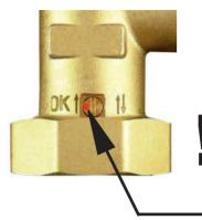
If the mark is on the left, the check valve is set to the position for normal operation. If you need to open the valve (e.g. to drain fluid from the system), turn the check valve control with the red dot to the right. This will deactivate the check valve function.
