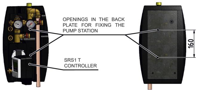
The supply involves an installation kit that is used to fix the pump station in its place.
