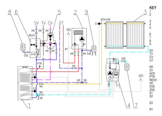
hot water storage tank boiler (el./gas/...) controlled by potential-free contact (cable included in pump station supply) solar collectors solar pump station pump station for DHW recirculation - CSE TVMIX ZV safety kit for HW storage tank solar expansion vessel DHW expansion vessel HC expansion vessel cold water
