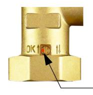
When the red mark is on the left-hand side, the non-return valve is set to normal operation position. If you need to open the valve (e.g. to drain the system), rotate its control so that the red dot is on the right-hand side. The non-return function is thus out of operation.
