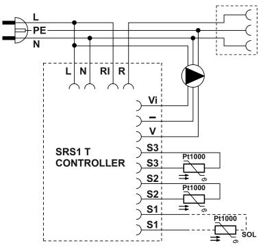
SPECIAL FEMALE SOCKET IN THE PUMP STATION, TO CONNECT AN EL. HEATING ELEMENT, UP TO 3 kW OUTPUT
