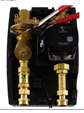
Remove the filter and mount the filter replacement section (code 19017) in its
