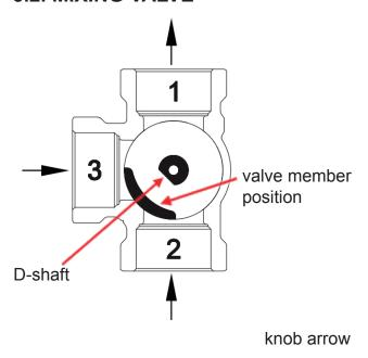
The knob arrow points always to the middle of the valve member. In this direction, the valve is closed.
