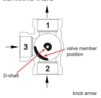
The knob arrow points always to the middle of the valve member. In this direction, the valve is closed.
