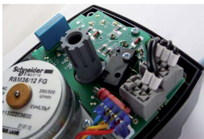
12. Remove the ring with shoulder for microswitch switching.
