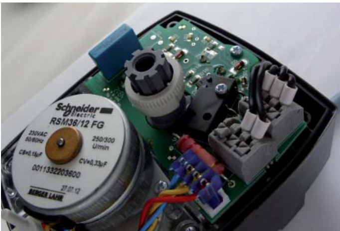
27. Remove the ring with shoulder for microswitch switching.
