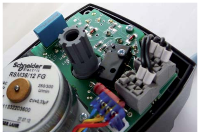
27. Remove the ring with shoulder for microswitch switching.
