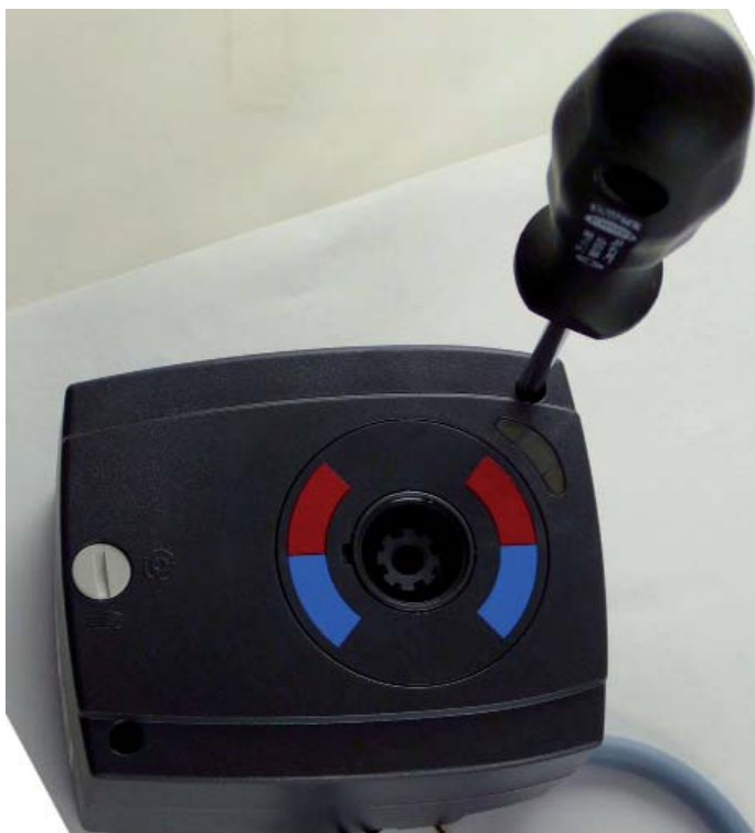
10. Unscrew two screws from the actuator body.
