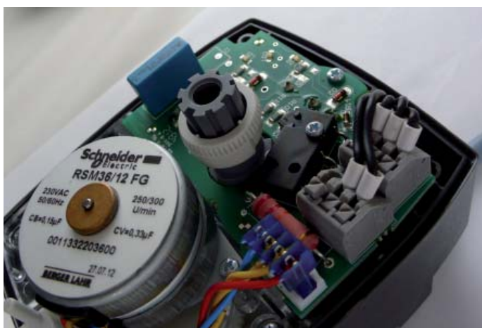
12. Remove the ring with shoulder for microswitch switching.
