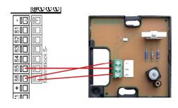
The switch changes the operation mode of the controller.
