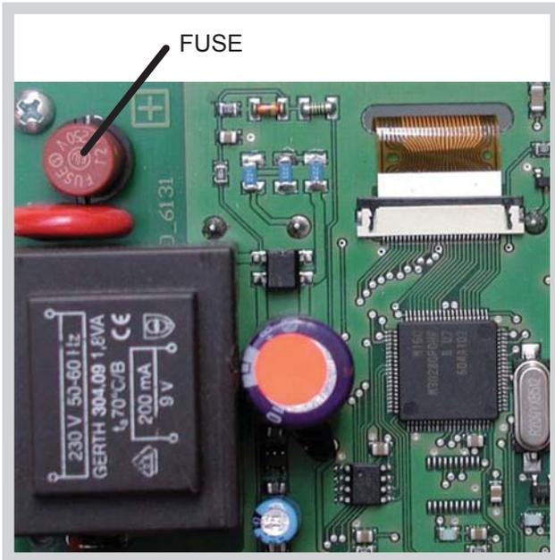
If the mains voltage is switched on and the controller still does not function or display anything, then the internal device fuse may be defective. In that case, disconnect the device, open it, remove the old fuse and check it. Replace the defective fuse with a new one, locate the external source of the error (e.g. pump) and replace it. Then first re-commission the controller and check the function of the switch outputs in manual mode as described in Chap. 3.2.
