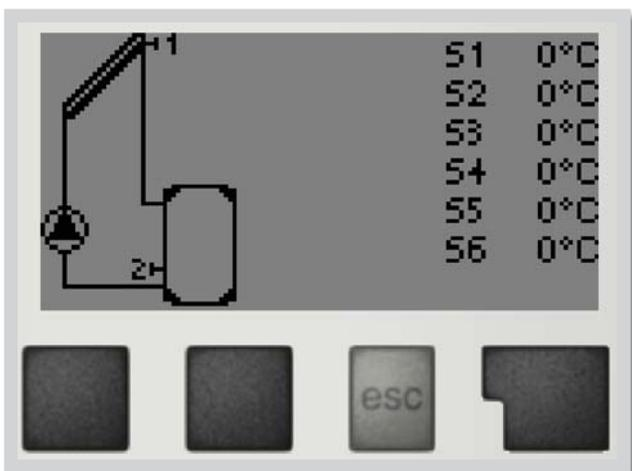
The graphics or overview mode appears when no key has been pressed for 2 minutes, or when the main menu is exited by pressing “**esc**”.
