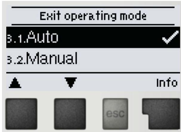
In menu “**3. Operating modes**” the controller can either be switched to automatic mode, turned off, or placed in a manual operating mode.
