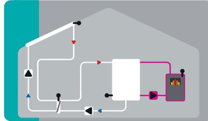
Solar with heat exchanger
