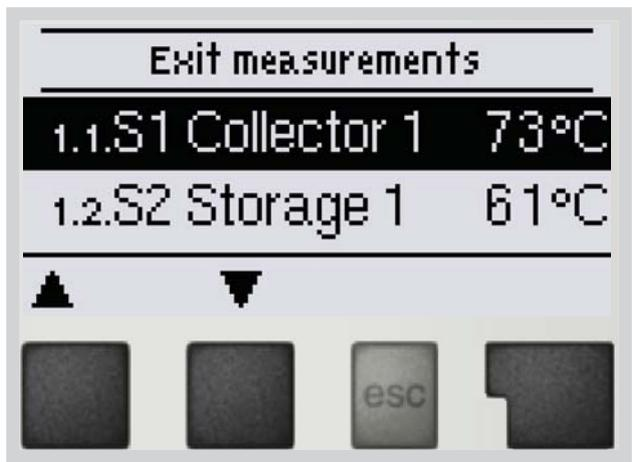
Menu “1. *Measurement values*” serves to display the currently measured temperatures.
