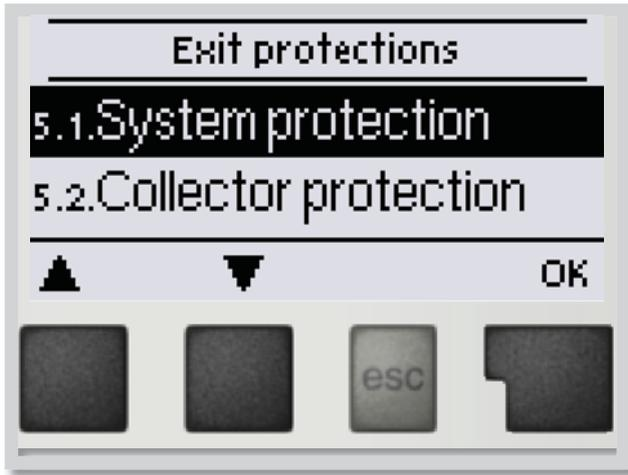
Menu „**5. Protections**” can be used to activate and set various protective functions.
