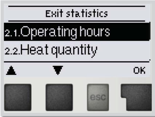
Menu “**2. Statistics**” is used for function control and long-term monitoring of the system.
