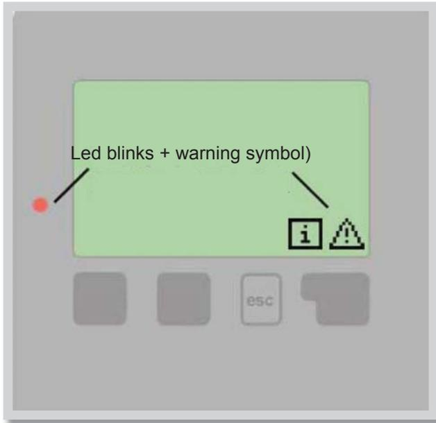
If the controller detects a malfunction or a non-standard system state, the red light flashes and the warning symbol also appears in the display. If the error is no longer present, the warning symbol changes to an info symbol and the red light no longer flashes.
