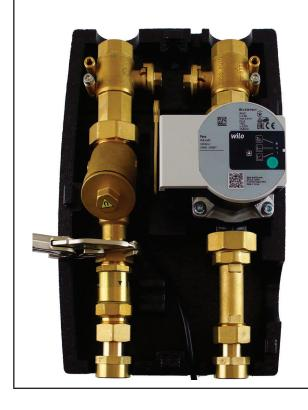
Loosen the union nut above and under Remove the filter and mount the filter replacement section (code 19017) in its place.
