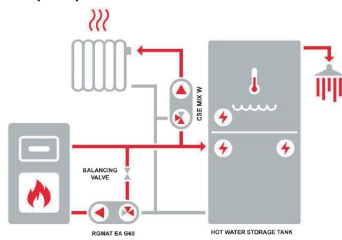
The diagram shows a typical connection of a solid-fuel boiler, combination thermal store and a heating circuit (with a recommended CSE MIX W pump station - not included in supply). A balancing valve shall be installed at the B inlet to the RGMAT EA W6 load unit.
