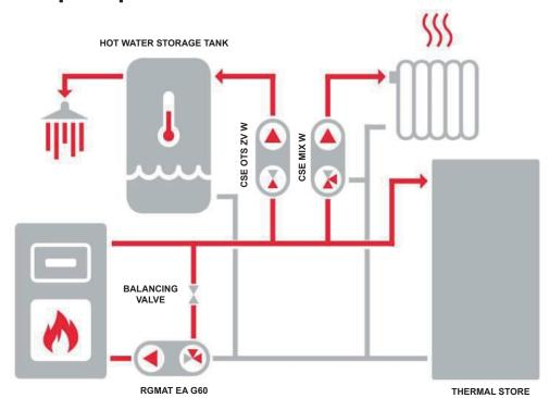
The diagram shows a typical connection of a solid-fuel boiler, thermal store and a heating circuit (with a recommended CSE MIX W pump station - not included in supply). If the boiler is also used for DHW heating, it is recommended to install also CSE OTS ZV W pump station (not included in supply). A balancing valve shall be installed at the B inlet to the RGMAT EA W6 load unit.
