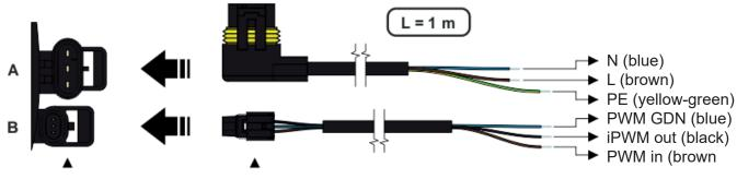
socket for power supply (A) and signal transmission (B)
