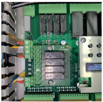
9. Remove the grey cable duct cover. There are such hooks that can be released by pushing in and prying out the plastic cover. The plastic can then be slid out all the way.
