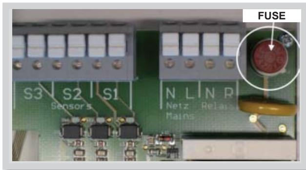
If the mains voltage is switched on and the controller still does not function or display anything, then the internal device fuse may be defective. In that case, disconnect the device, open it, remove the old fuse and check it.
