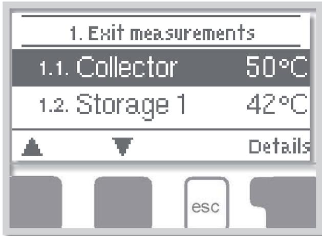
Menu „**1. Measurements**” serves to display the currently measured temperatures. The menu is closed by pressing „**esc**” or selecting „**Exit measurements**”.
