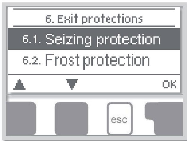
Menu „**6. Protections**” can be used to activate and set various protective functions. These functions do not under any circumstances replace safety elements in solar systems!
