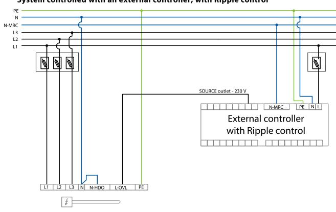
System controlled with an external controller, with Ripple control
