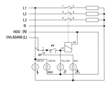
2.4.1.2 - Heating rods 7.5 - 9 kW
