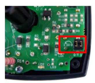
3. In the factory setting, the jumper is placed vertically. The actuator turns clockwise.
