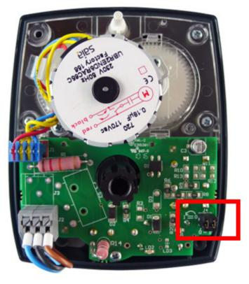
1. Switch off the supply voltage, set the manual control, unscrew and remove the actuator cover.
