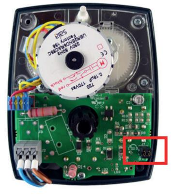
1. Switch off the supply voltage, set the manual control, unscrew and remove the actuator cover.
