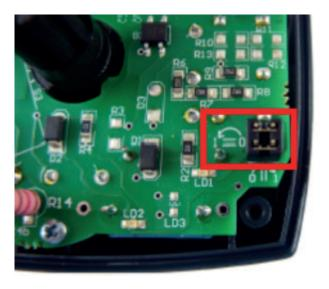
4. Turning the jumper by 90 deg. to the horizontal position will change the direction of rotation. The actuator now turns anti-clockwise.
