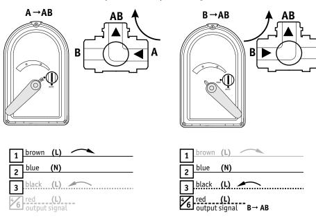
opens. When the terminal 3 (black wire) is energized, the actuator turns counterclockwise, i.e. the path B-AB opens. As soon as the path B-AB fully opens, 230V tension appears on the terminal 4/6 (red wire).
