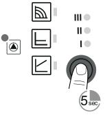
If the pump has been inactive for a long time or is blocked, activate the manual restart by holding the operating button for 5 seconds. The LEDs flash sequentially clockwise. The manual restart takes max. 10 minutes before the pump returns to normal operation. To cancel the manual restart, hold down the operating button for 5 seconds.
