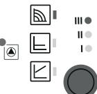
Briefly press the operating button for 1 second to select operating mode and pump performance curve. LEDs show pump settings (operating mode / performance curve).
