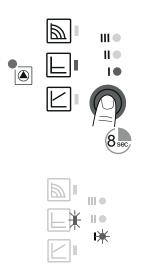
To lock the operating button, press it for 8 seconds.
