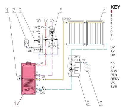
RDC hot water storage tank CSE SOL solar pump station solar expansion vessel solar collectors pump station for DHW recirculation - CSE TVMIX ZV safety kit for HW storage tank DHW expansion vessel el. heating element cold water hot water hot water recirculation ball valve check valve automatic air vent valve pressure temperature relief valve
