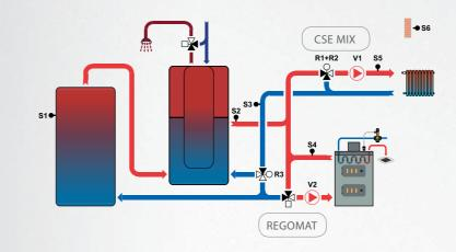
CSE MIX (G or W PWM) – insulated pump station with a circulation pump and a heating circuit mixing valve. **REGOMAT E (G or W PWM)** - insulated load unit with a circulation pump and a solid-fuel boiler thermostatic valve.
