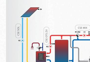
**CSE MIX (G or W PWM)** – insulated pump station with a circulation pump and a heating circuit mixing valve. CSE OTS ZV (G or W) – insulated pump station with a circulation pump, non-return valve and two ball valves. CSE SOL - insulated solar pump station.
