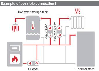
The diagram shows a typical connection of a solid fuel boiler (with the recommended RGMAT pump station – not included in supply), thermal store and heating circuit. If the boiler is used also for hot water heating, it is recommended to install a CSE OTS ZV W pump station (not included in supply).
